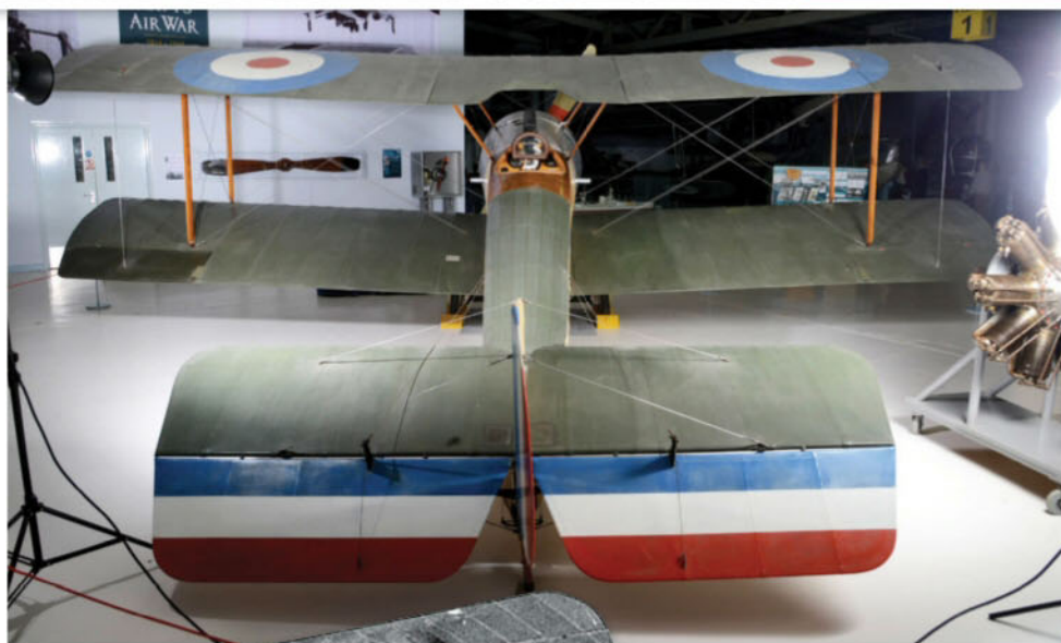
Right: A single-seat fighter, the Pup had a wooden frame covered in canvas
